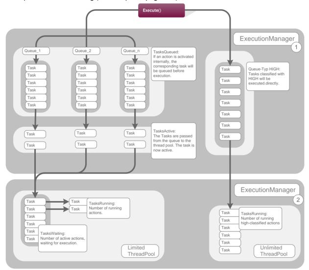
Figure 9-6: Execution of tasks using the ExecutionManager
