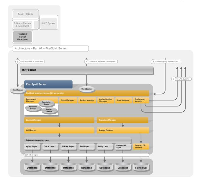
Figure 1-3: Total architecture – Detail: FirstSpirit Server
